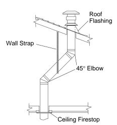
Figure 21 - Offset with Wall Strap and 45° Elbows
